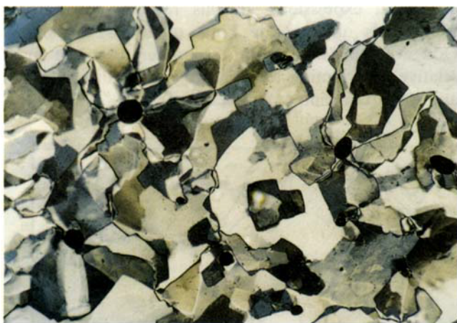
Figure 8. Smectic S 2 phase of 10OTO6OTO10 at 172.6°C (the same sample, cooling, crossed nicols, \times 225 ).
