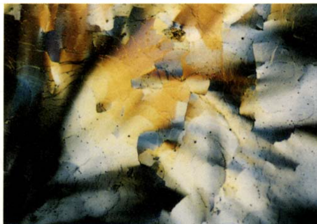
Figure 11. Smectic S 2 phase of 14OTO6OTO14 at 161.4°C, the same sample after rotating of nicols by 30° clockwise (cooling, crossed nicols, \times 225 ).
